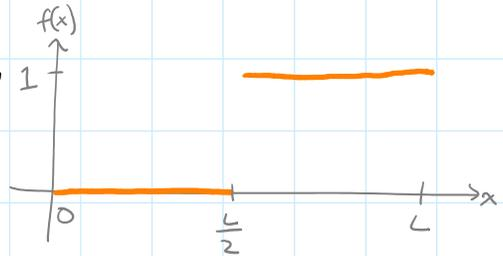
and:  $A_0 = \frac{1}{L} \int_0^L f(x) dx = \frac{1}{L} \left( \int_0^{\frac{L}{2}} 0 dx + \int_{\frac{L}{2}}^L 1 dx \right) = \frac{1}{L} \left( 0 + \frac{L}{2} \right) = \frac{1}{2}$
