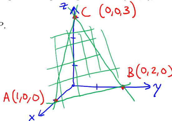
(b) One vector parallel to the plane is  $\vec{AB} = \langle -1, 2, 0 \rangle$ . A different vector parallel to  $P$  is  $\vec{AC} = \langle -1, 0, 3 \rangle$ . How can you find a vector  $\mathbf{n}$  that is *perpendicular* to the plane  $P$ ?
